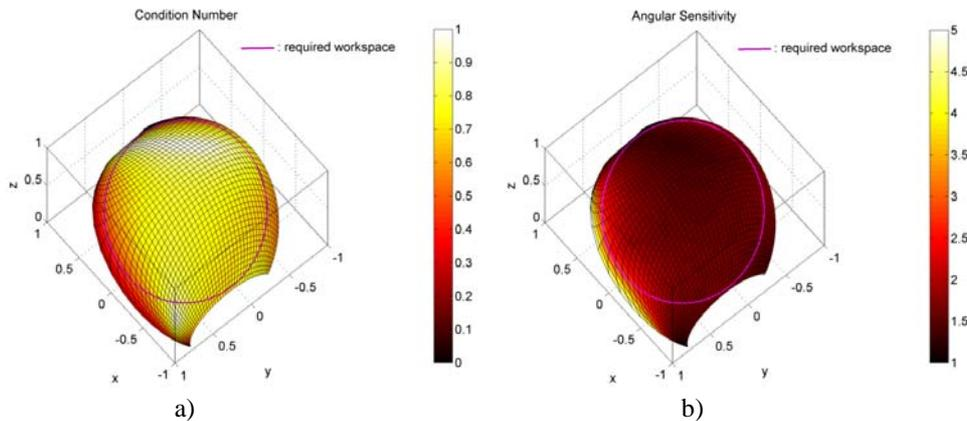
Figure 5: a) Condition Number over the workspace; b) Angular sensitivity (ratio between encoder resolution and platform global rotation angle) over the workspace.
